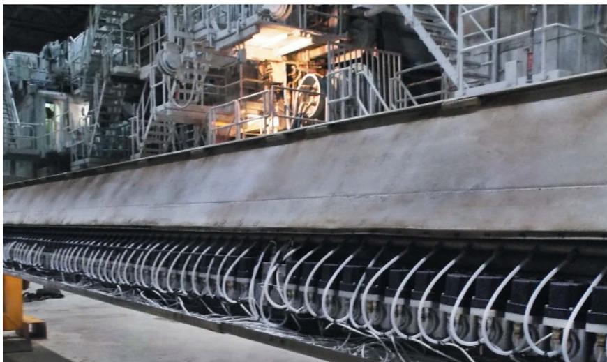
The profiler has 114 new actuators.
