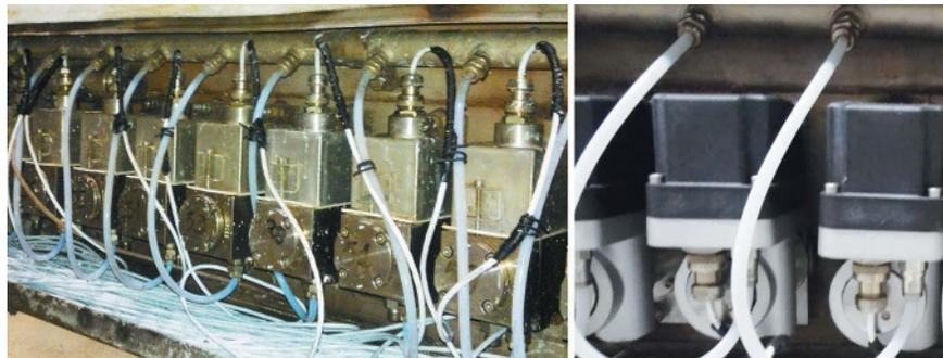
Original actuators (left) and new STA-1015 actuators (right).
