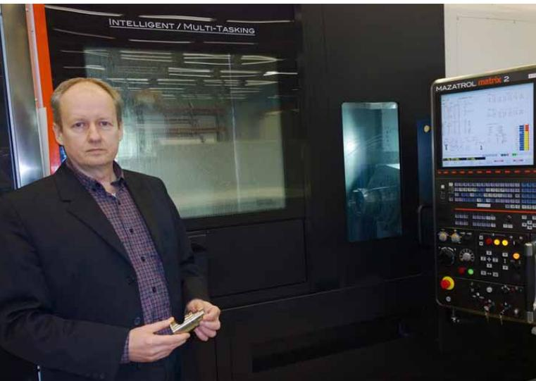
*Tasowheel Systems produces the core parts for the actuators and valves in the company's factory in Tampere, Finland. "We invested heavily last year in a modern multi task CNC lathe, that carves the components directly from the extremely hard stainless steel bars", says Jukka Ahlstedt, Sales Manager at Tasowheel Systems. © Tasowheel*
