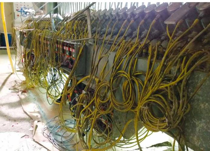
*The heap of separate cables around the old set of actuators was eliminated in a paper machine that recently was fitted with a new set of Tasowheel Systems' CD actuators, which connect directly to the CD profiling system's I/O control cards.*
