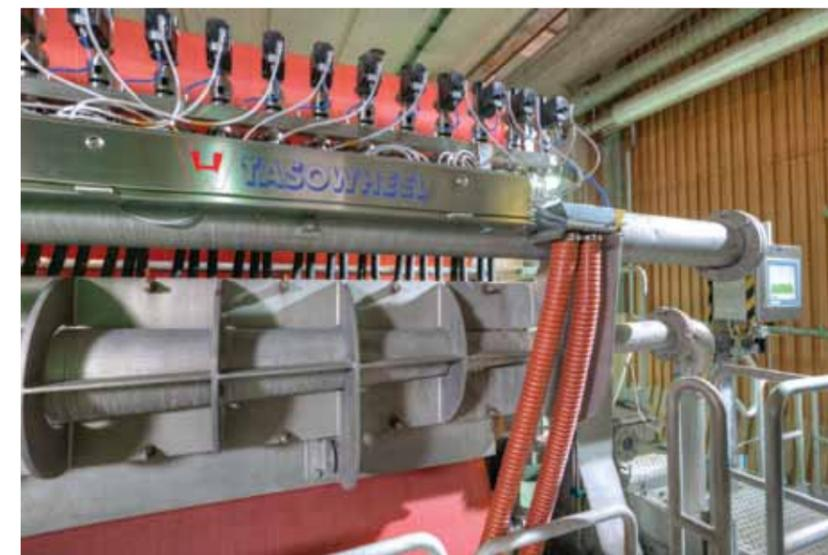
The dilution water valves delivered by Tasowheel have no plastic parts.
